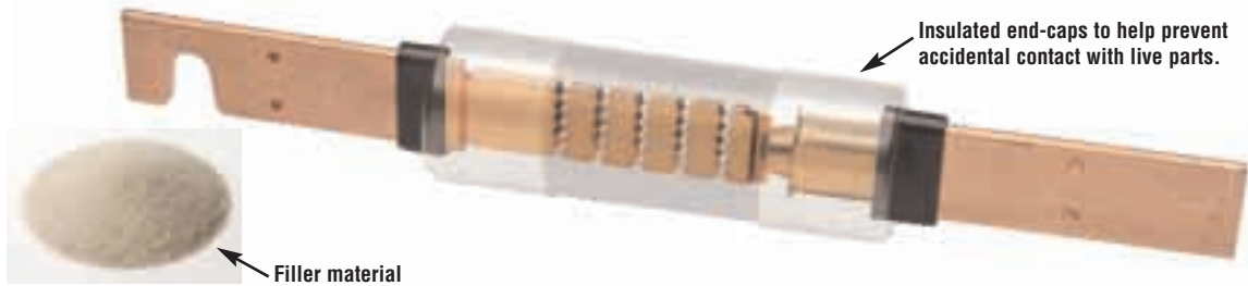
Figure 6. This is the LPS-RK100SP, a 100A, 600V LOW-PEAK®, Class RK1, Dual-Element Fuse that has excellent time-delay, excellent current-limiting and a 300,000A interrupting rating. Artistic liberty is taken to illustrate the internal portion of this fuse. The real fuse has a non-transparent tube and special small granular, arc-quenching material completely filling the internal space.
